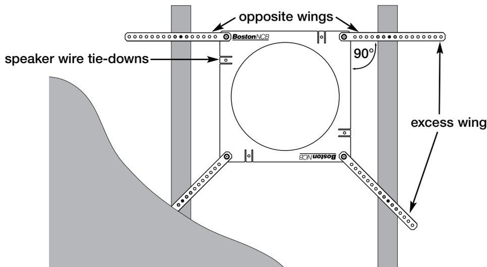
\*Behind the wall there must be 1 inch (25.4mm) clearance around the mounting hole.
