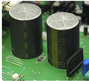
Robust, high-speed power supply (with blocking capacitors and large-capacity Schottky Barrier Diodes)
