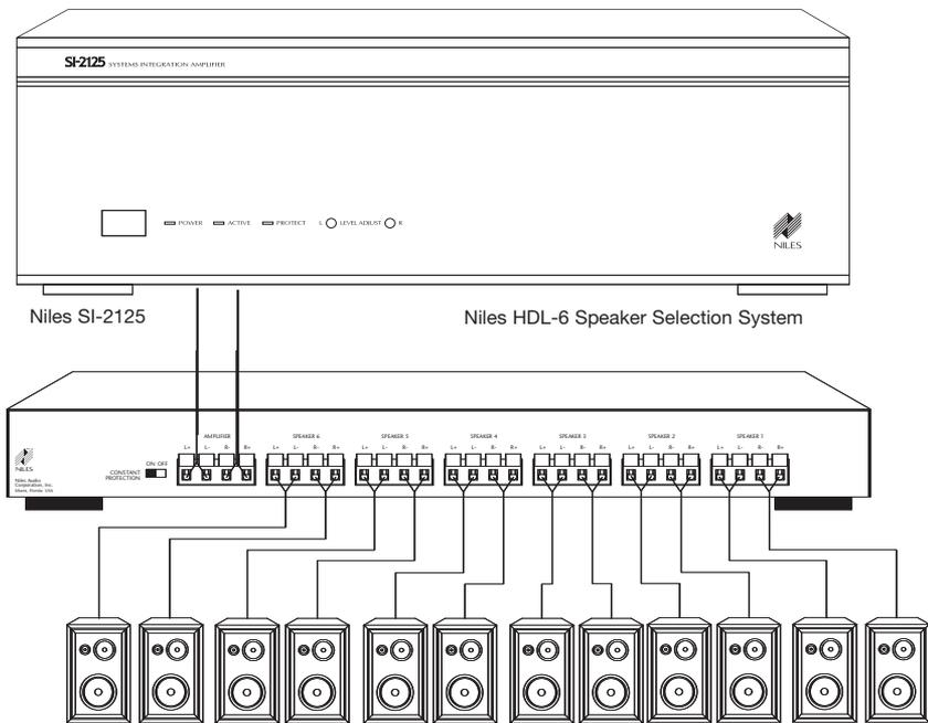
Speaker selection systems allow each pair of speakers to be turned on and off from your equipment location (or even via remote control).
