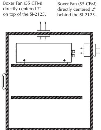
If the cabinet rear is not open to fresh air or if you're using low impedance loads, install two "boxer fans" to provide continuous air flow into and out of the cabinet.
