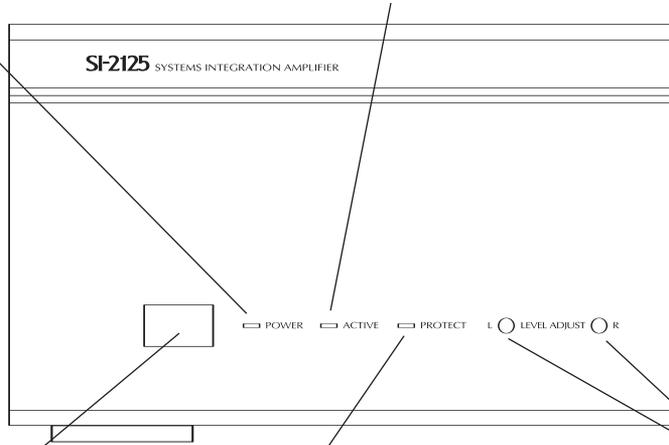
Front panel "Master Power" switch turns off the entire amplifier, including the Turn-On circuitry.
