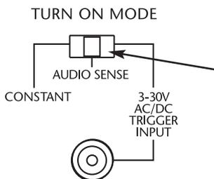
Slide the switch with your fingernail or a 1/8" slotted screwdriver blade.
