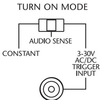
**Constant** - The auto turn-on circuitry is off. The front panel master power switch operates the amplifier. In is "On", out is "Off".
