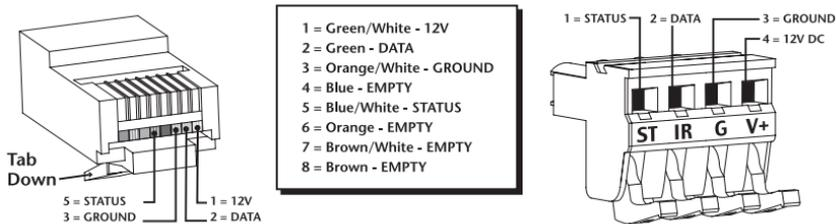
**Figure 4** This color code is based on the industry standard T568A coding for the RJ45 connector. When connecting the WS120 to the Niles MultiZone Keypad that have IR-Sensor connection observe this pin configuration.
