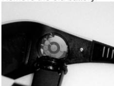
4. Insert the new battery inside the compartment.
