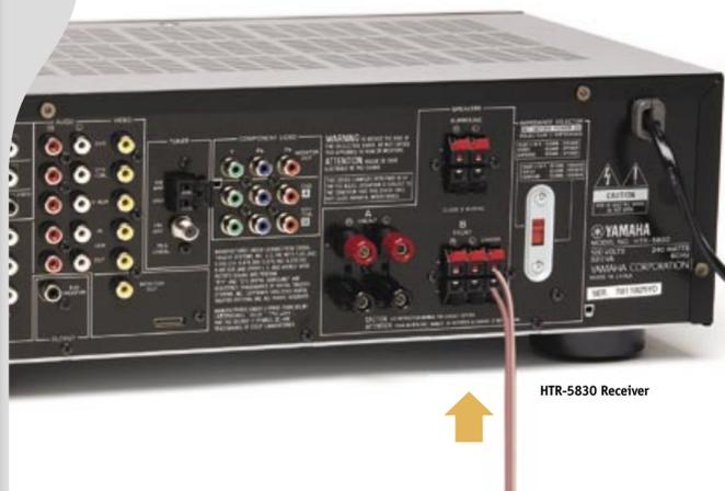
**Connect Center Speaker** Positive (+) side of the wire with white stripe attaches to (+) terminal. Negative (-) side attaches to (-) terminal.
